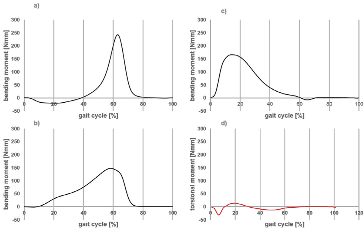
**Figure 2** Characteristic loading curves of a) bending moment at MTP I, b) bending moment at DI, c) bending moment at heel and d) torsional moment at heel. Positive bending moments indicate dorsal extension and negative plantar flexion. Positive torsional moments indicate an eversion and negative an inversion.
