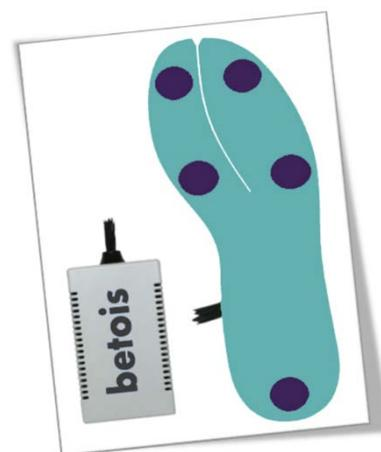
**Figure 1 betois (bending torsion insole system) system with five measuring points and A/D- converter.**
